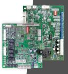
7. Aurora Controls: The powerful Aurora Base Control (ABC) offers two way communication between components, advanced operating logic and robust troubleshooting capabilities. The Aurora Expansion Board (AXB) adds support for true energy monitoring as well as compatibility with the Symphony Home Comfort Platform and our IntelliZone2 zoning system.
